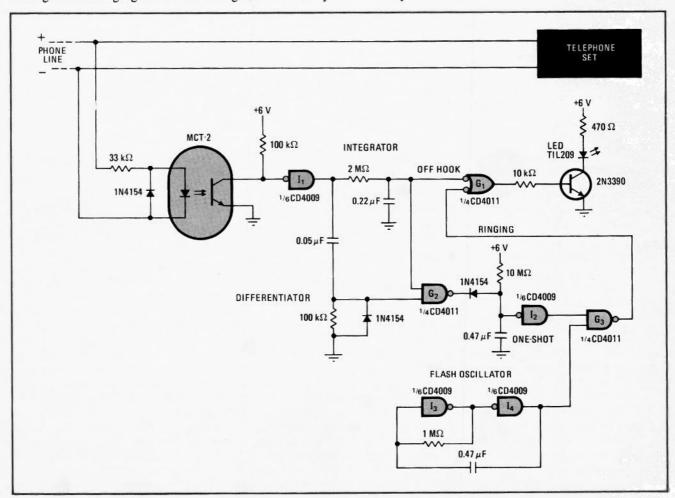
**Secretary's helper.** LED indicates status of a remote telephone. Light is off if phone is hung up, shines steadily if phone is off hook, and flashes on and off while phone rings and for 5 seconds after ringing stops. The flashing oscillator operates continuously, but can drive LED only when a ringing signal discharges the one-shot capacitor to enable NAND gate G<sub>3</sub>. Thus, one oscillator handles several phone lines.
